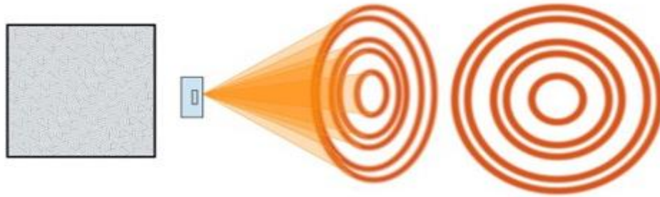
Figure 45: Diffraction of an ideal powder (uniform intensity around the diffracted rings)
