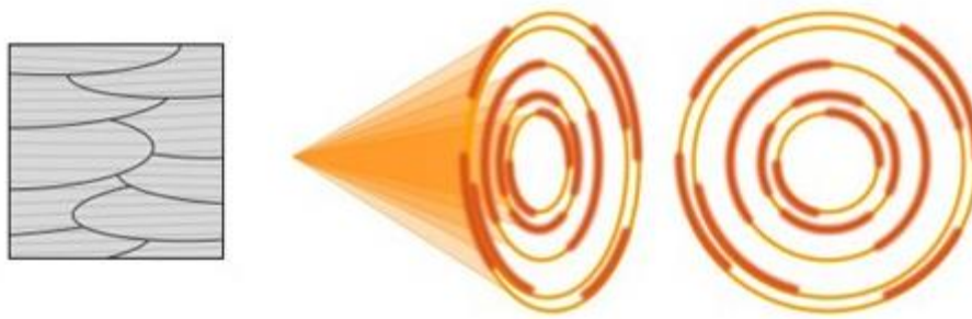
Figure 47: Diffraction from textured samples (the degree of orientation can be extracted)
